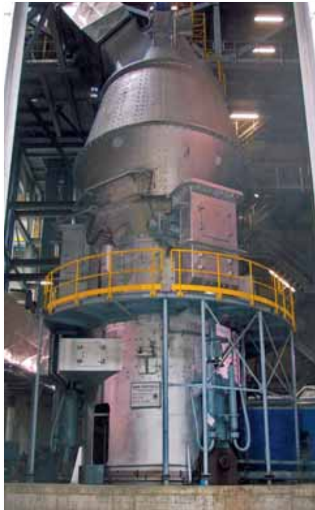
Figure 4: View of the MPS 4250 BC vertical roller mill at the Merone cement works in Italy
