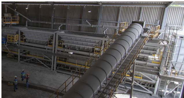
Figure 6: Feed bin (A. 1) with optional pre-feed system (B. 7) of the ready2grind plant in Caldera
