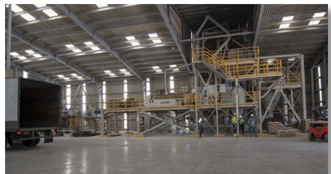
Figure 8: Packing and palletizing plant (B. 2 and B. 3) of the ready2grind plant in Caldera
