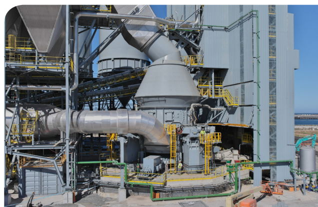
Figure 2. Pfeiffer MVR 6000 C-6 vertical mill with MultiDrive®.
