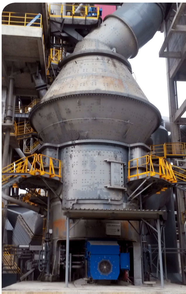
Figure 1. MPS 4500 BK, the world's largest coal mill, producing for Semen Merah Putih in Bayah.
