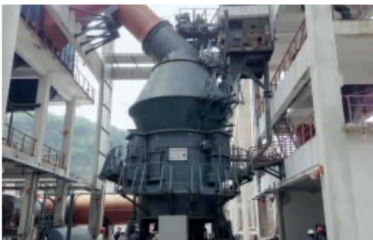
Grinding of limestone with MPS 3350 B in China
