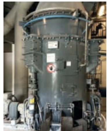
Quicklime grinding with MPS 200 B in Bulgaria
